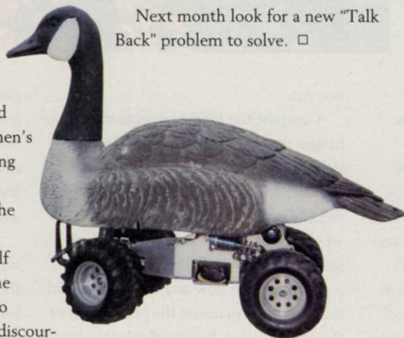
Jim Carpenter's Barberton, Ohio, crew constructed a radio-controlled 'Robo Goose' on a toy car chassis.
