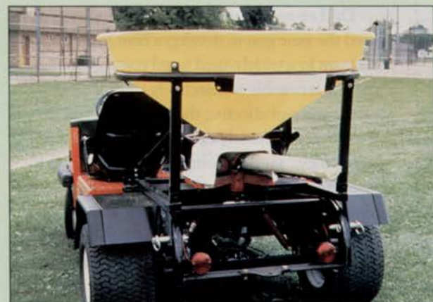
Jacobsen's SV System Vehicle with spreader attachment. The spreader carries 14 cubic feet of material.
