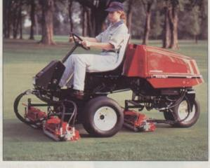
The Greens King V is powered by a 19 hp Kubota diesel, or high output 18 hp Briggs & Stratton Vanguard gas engine—take your choice.
