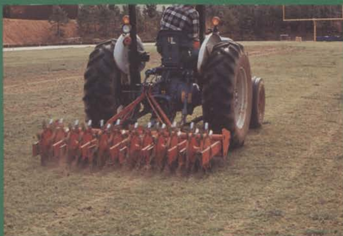
Verticutting fields helps control thatch and compaction caused by high use and heavy athletes.
