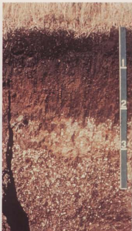
Fig. 4 —At least 12 inches of rich organic matter ("A" horizon) is desirable to support turf and tree growth.
