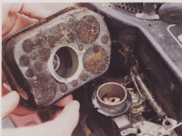
A dirty air filter also keeps air from getting to the engine and affects the air-fuel ratio.
