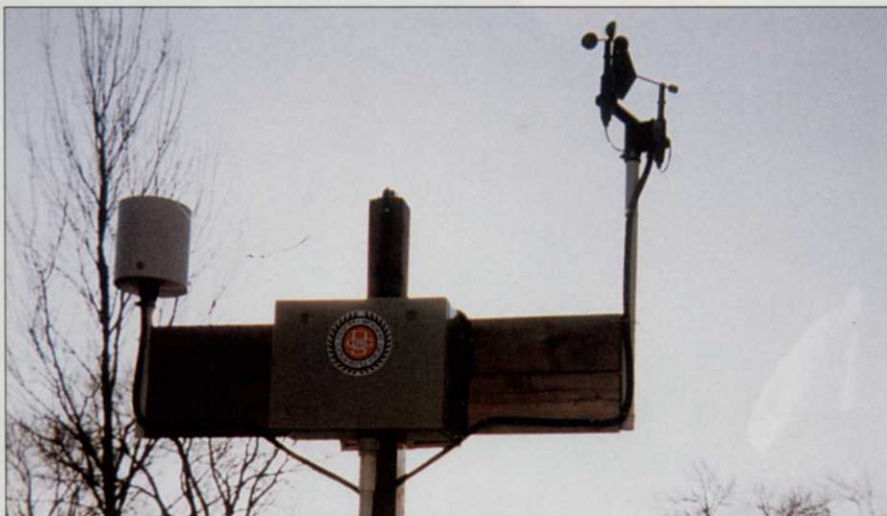
The Metos weather station references evapotranspiration rate as inches or millimeters of water loss per 24-hour period.
