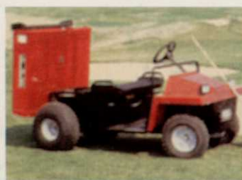
Haulmaster with 16 hp engine
