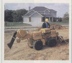
The vibratory plow attachment features a shaker box that delivers 10,000 lbs, of force to the plow for more efficient plowing and increased productivity.
