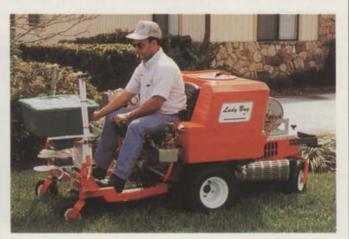
The rear wheel can be removed to allow for quick engine checks, and the front tilts down to allow inspection of hydro units, belts or battery.
