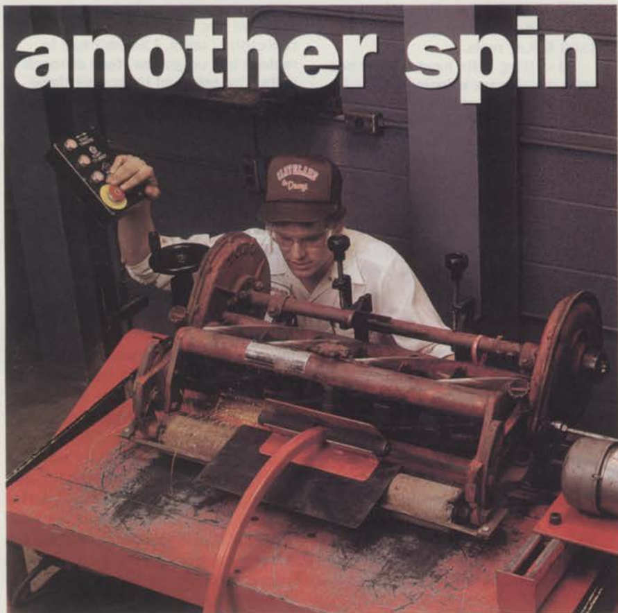
On greens mowers and walkers, the most often used grinding angle is 7° plus a 'dirt factor' of 2°.
