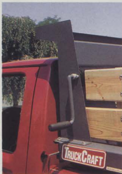
Truck Craft's TC-100 pickup dumper features a rear window protector.
