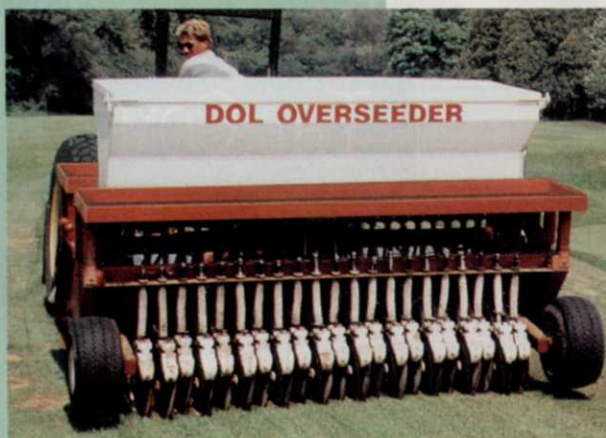
Overseeding, pesticide injection or fertilizing can be done with the Dol overseeder.
