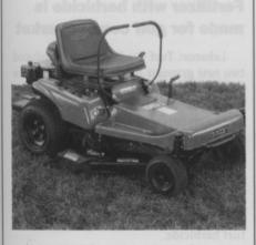
The 2301 features a 30-inch cutting deck, compact design and zero turning radius mobility which allows the operator access to areas previously only mowed by walk-behind mowers.
