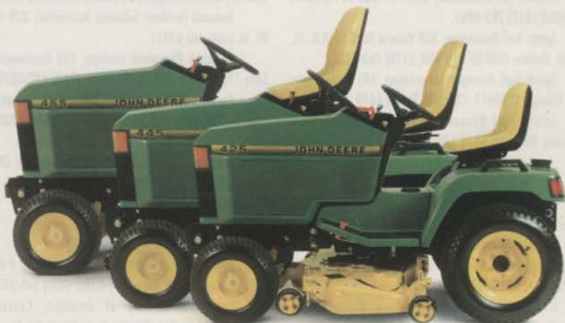
The 400 Series Tractors: 20-hp 425, 22-hp EFI 445, and the 22-hp, diesel 455.
