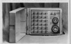
The unit combines electromechanical and micro-electronic circuitry. It is capable of fully automatic, semi-automatic or manual operation. All of the programming is through user-friendly dial or lever switches and push/pull pins.
