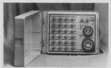
The unit combines electromechanical and micro-electronic circuitry. It is capable of fully automatic, semi-automatic or manual operation. All of the programming is through user-friendly dial or lever switches and push/pull pins.
