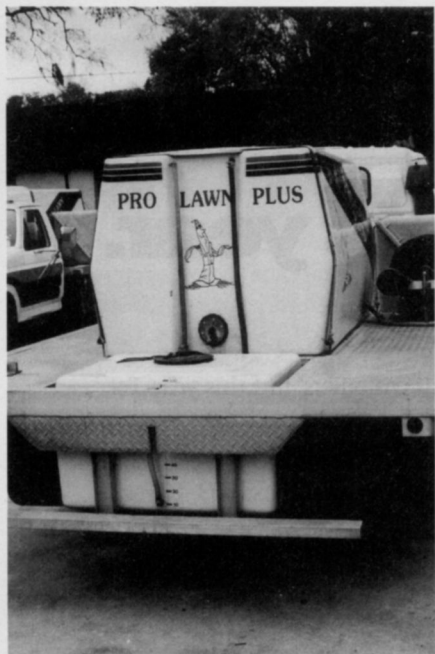
Pro Lawn Plus is using Isuzu trucks this season with 600 gallon main, 100 gallon drop tanks.
