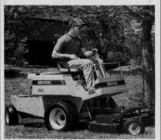
drive wheel motors. According to Excel, the drive concept eliminates the need for high maintenance chains, sprockets and transaxles.
