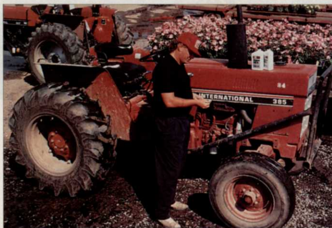
Checking the oil at three-hour intervals keeps Bailey's tractor fleet always ready to do the toughest jobs.
