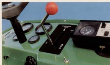
A single lever hydrostatically controls the 1800's direction and speed.
