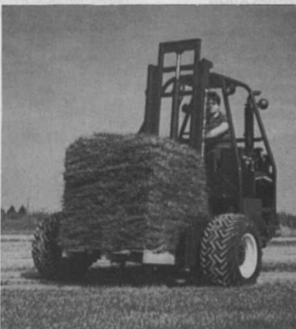
The 60-inch-wide Piggyback can carry loads from 3,000 lbs. up to 5,500 lbs.
