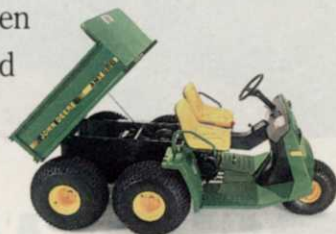
Hydraulic dump option on the AMT 626 allows you to empty its cargo box from your seat.
