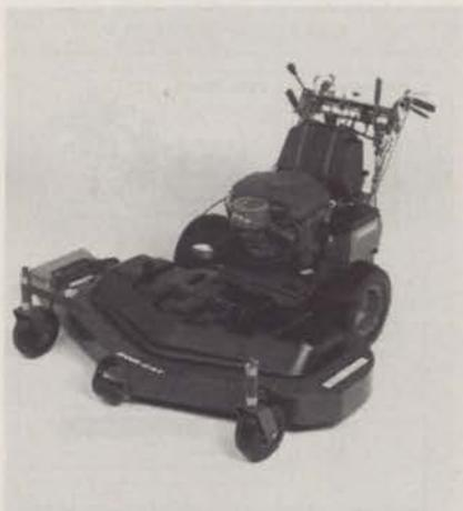
ers. Ransomes believes the hydrostatic system offers improved performance and eliminates the hassles commonly associated with belt-driven mowers.
