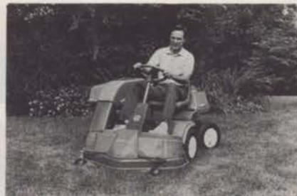
The front-mounted blade empties into a side-mounted bagging unit which houses two six-bushel containers.
