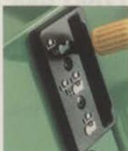
Just a flip of a lever lets you choose which implement to run. Separate and simultaneous PTO selection levers let you go from mowing to tilling without removing implements.
