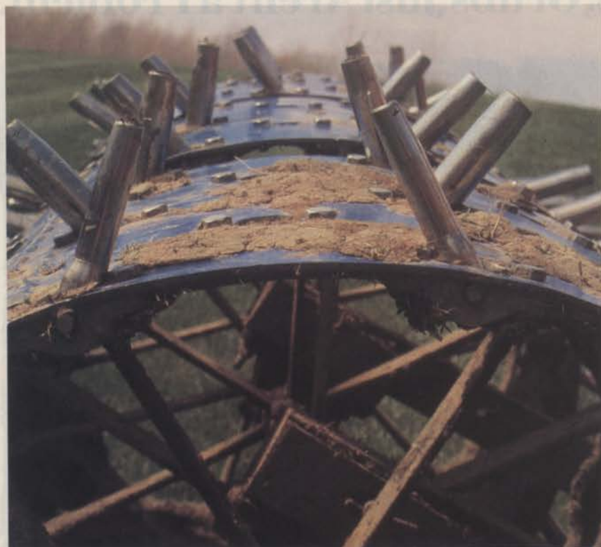
The old standby drum roller, which aerates quickly and never needs fueling. Drums can be detached, depending on the size of the area in question.
