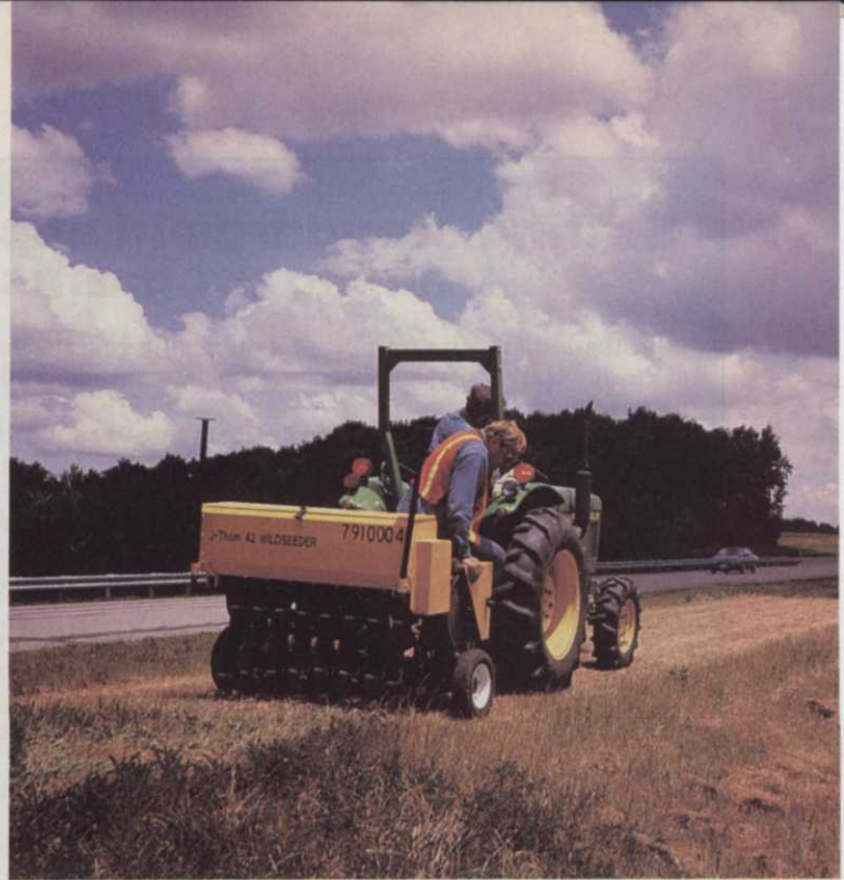
The Ohio DOT uses this no-till seeder to plant wildflowers.
