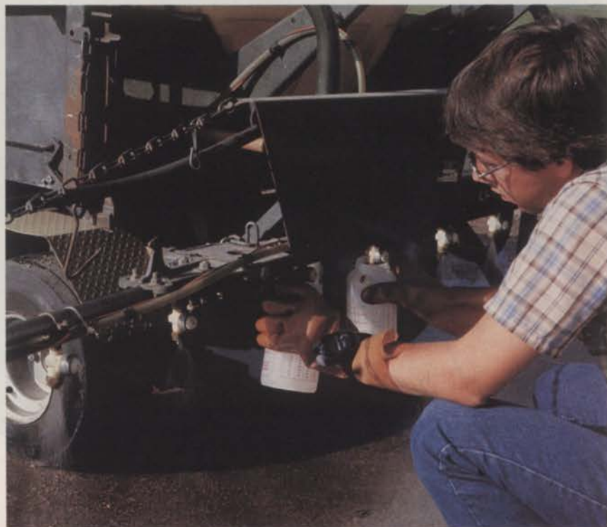
Frequency of sprayer calibration was found to be closely associated with application accuracy. Two-thirds of the applicators who calibrated before each spray operation were delivering within five percent of their intended amount.
