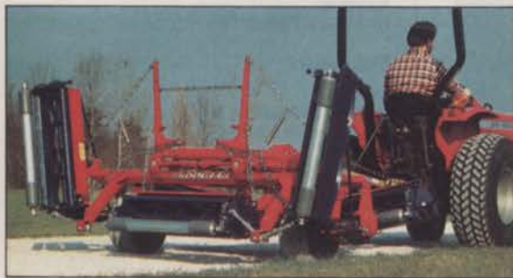
2. Hydraulic lift for easy transport or storage
