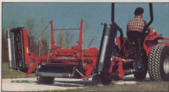
2. Hydraulic lift for easy transport or storage
