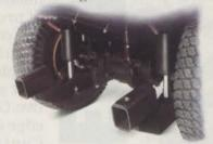
John Deere front mower implements can be attached or removed by one person in minutes. Four pins attach the implement securely to dual lift cylinders.
