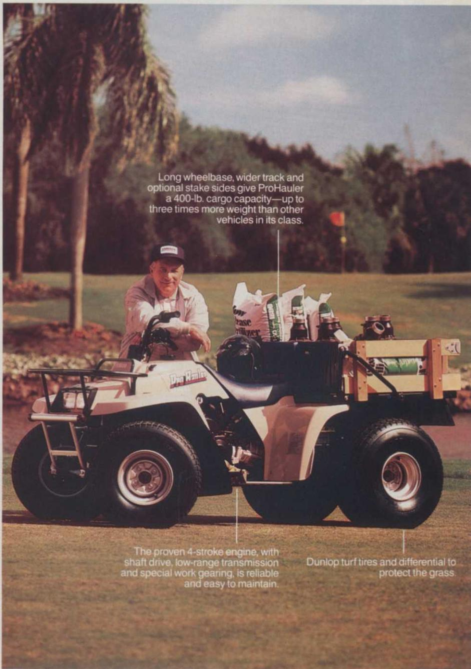
Long wheelbase, wider track and optional stake sides give ProHauler a 400-lb. cargo capacity—up to three times more weight than other vehicles in its class.
