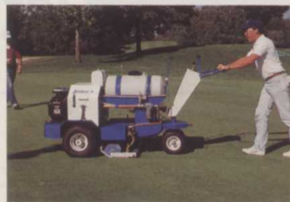
The RainSaver Jr. opens the turf with coulters before material is sprayed in.
