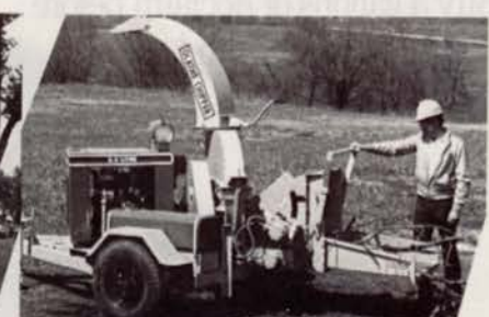
Model 986 — Hydraulic feed disc chipper features: 12" capacity, variable feed rate, gas or diesel, and 15° curbside feed angle for safety.
