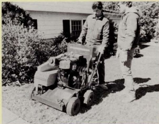
Vertiseeding mixes the humus and soil, creating the optimum environment for germination.
