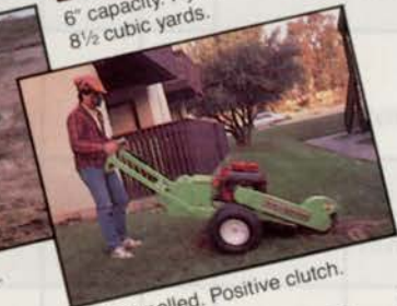
Full vision cutting, 22" wide. Hydrostatic drive.
