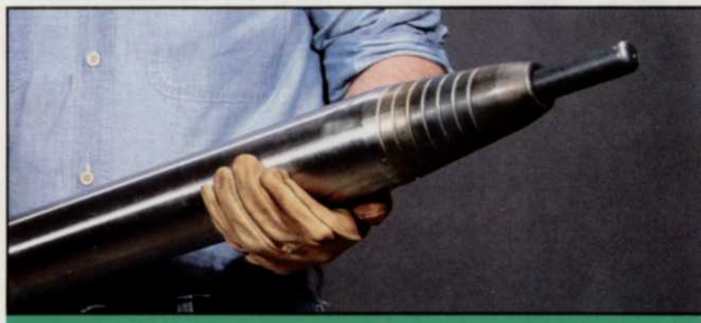
The versatile Pierce Airrow tool installs pipe, cable or wire under obstacles where other methods are cost prohibitive.
