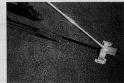
vandalism. It cuts out the damaged sod and replacement strips. Available in three, five and seven inch sizes.
