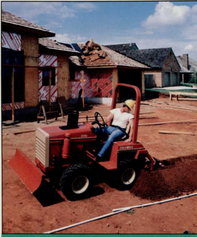
The 2310 has an enclosed gearbox, which eliminates driveline adjustments.
