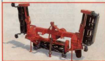
Rear mower assembly detached
