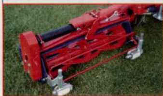
Fixed cutting unit, with anti-scalp rollers.
