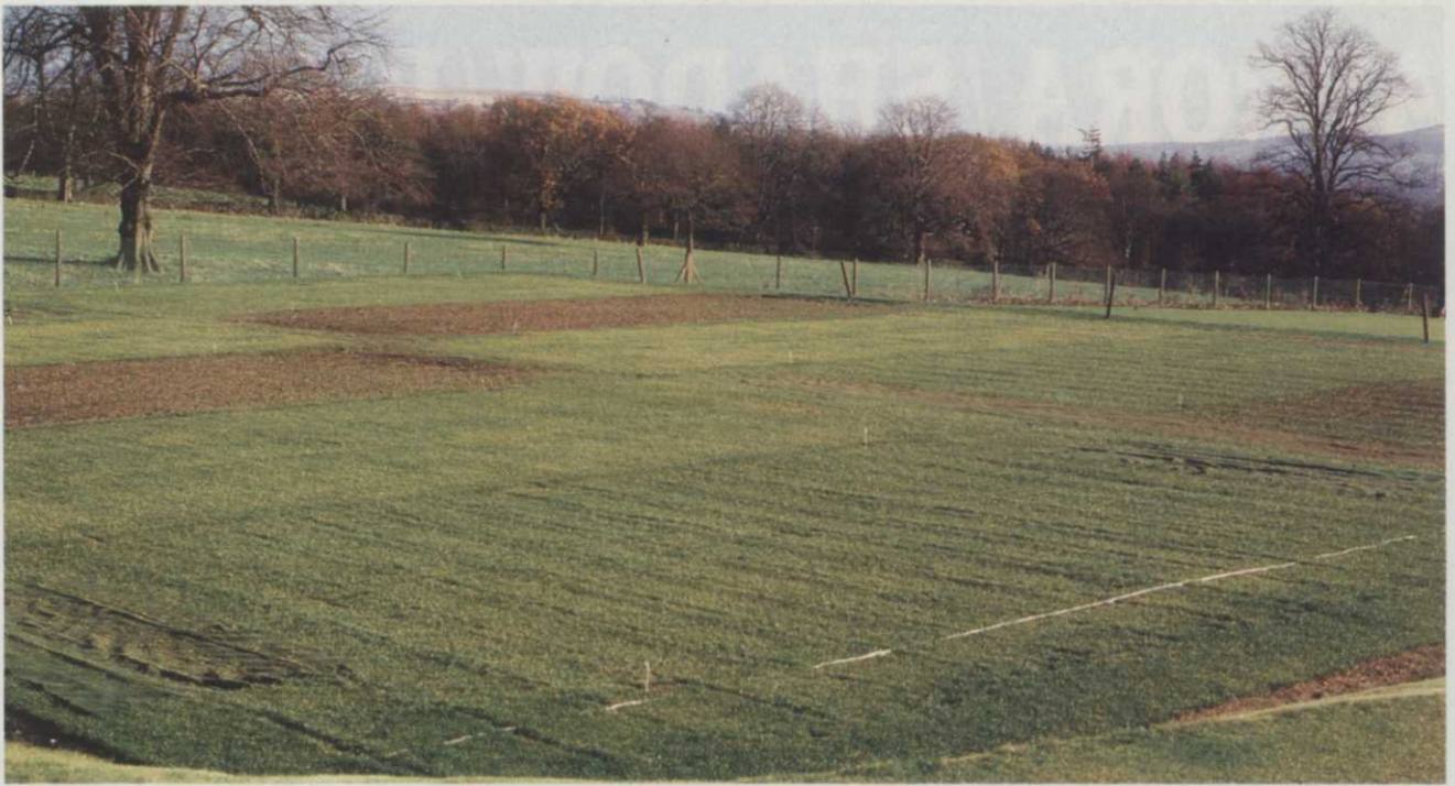
A trial at the Sports Turf Research Institute shows the cost-effectiveness of different construction methods. The same intensity of simulated wear is applied to all plots, but those with pipe drainage are a sea of mud, while the slit-drained and sand rootzones retain a good grass cover.
