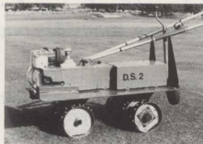
A differential wear machine is fitted with studded rotors to simulate football-type wear.
