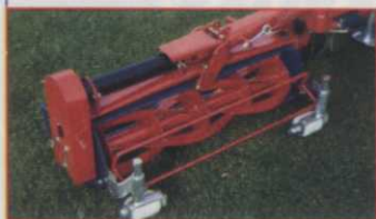
Fixed cutting unit, with anti-scalp rollers.
