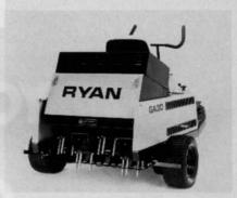
The throttle, choke and ignition switch are also hand-operated while speed, brakes and lift control for the aerating head are controlled by foot pedals. The machine has hydrostatic drive, and transport speed is 6 mph, nearly double that of other aerators.
