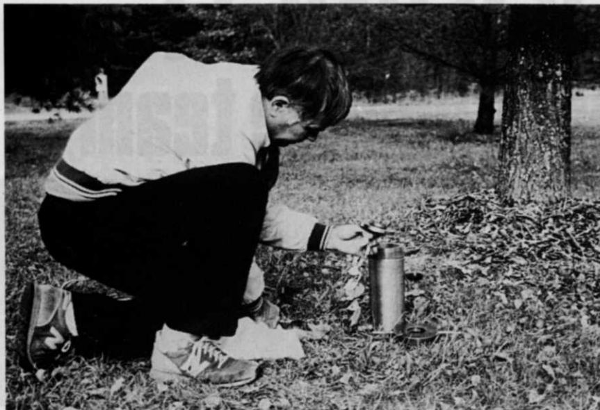
Measuring the water status of woody plant tissue using the pressure equilibration technique.
