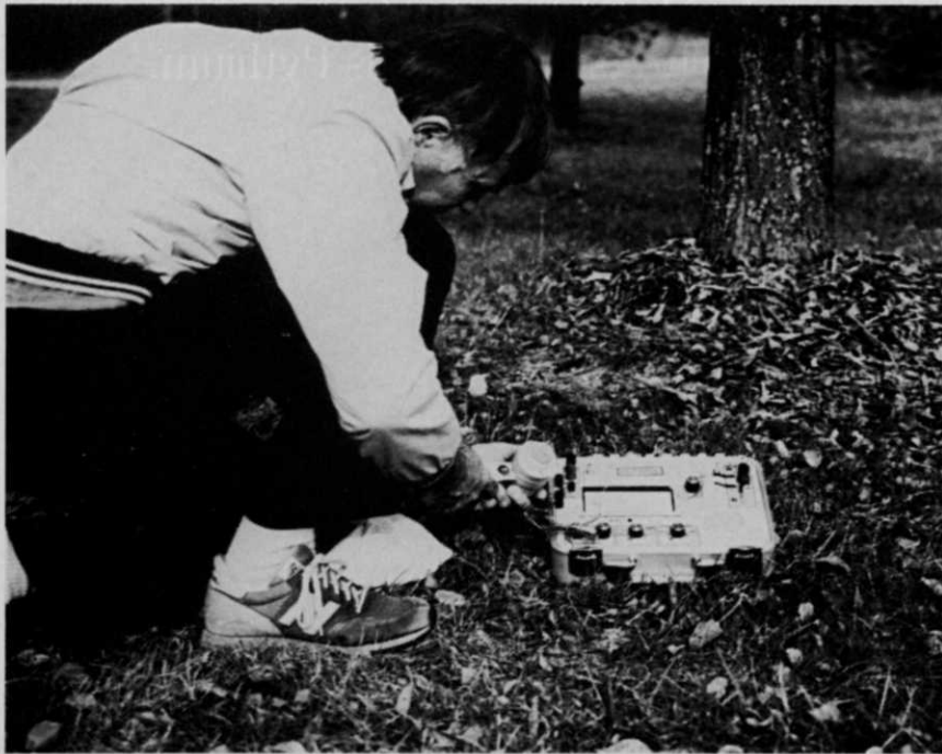
Measuring the water status of woody plant tissue using the thermocouple psychrometer technique.
