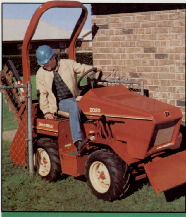
The 2020 can go through a 36-inch yard gate to enter backyards or other confined jobsites.
