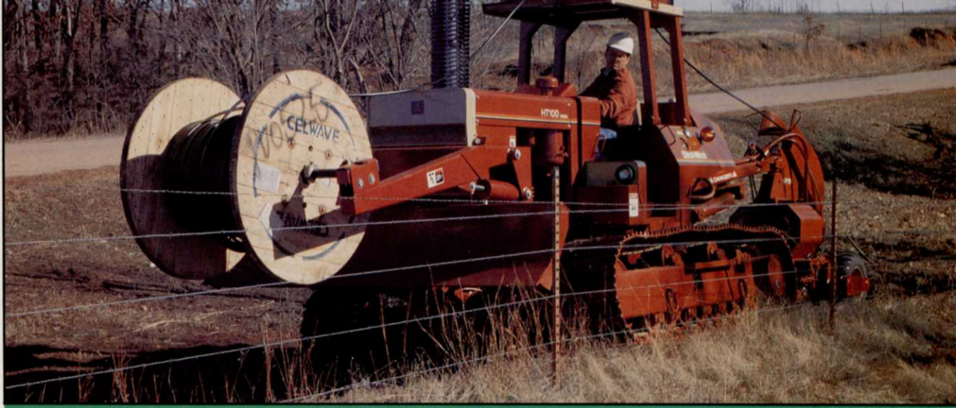
The HT100 is a 100-HP-class track machine that can either be a vibratory plow, trencher or earth saw.
