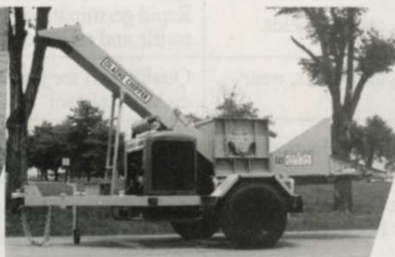
Model 816 — Debris chipper handles kiln dried lumber and assorted wood debris.
