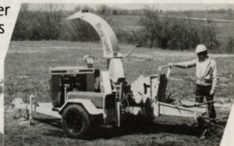
Model 986 — Hydraulic feed disc chipper features: 12" capacity, variable feed rate, gas or diesel, 360° swivel chute, 15° curbside feed angle for operator safety, over 950 RPM drum speed. Compare! Olathe wins!
