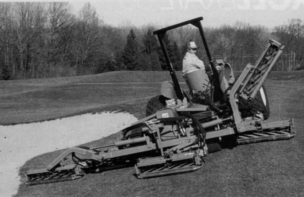
Reel mowers, like this Jacobsen five-ganger, are perfect for golf course fairways.
