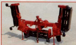
Rear mower assembly detached
