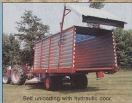
Self unloading with hydraulic door.
