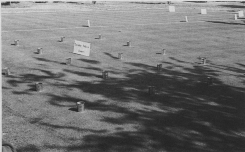
Cans set out in a grid pattern on a golf green help evaluate the distribution uniformity of the irrigation system.
