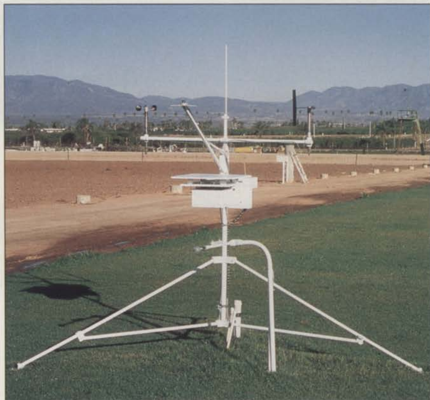
This automatic weather station reports local evapotranspiration information as part of a statewide system in California.
