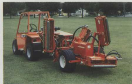
Jacobsen's new Five-Gang Hydraulic Ranger swings up quickly to a compact 7' transport width, and large 26" high-flotation tires move softly over fine turf.
