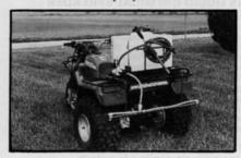
diaphragm pump, a pressure gauge and a heavy-duty toggle switch directly behind the operator's seat.
