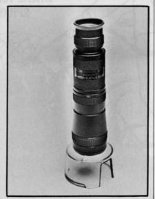
SLR cameras, permitting photomicrography at 18 to 36 times magnifications in the field at a nominal cost without elaborate set-up.
